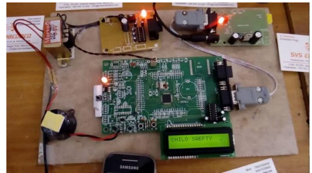
Fig.10.Hardware implementation of SMS sending
