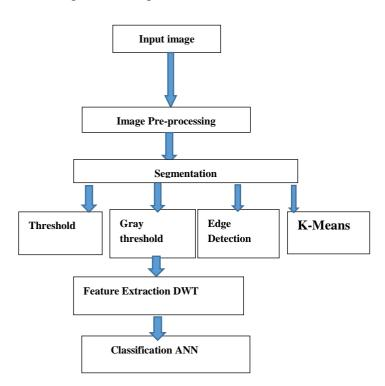
Fig (1) Block Diagram of the proposed system
