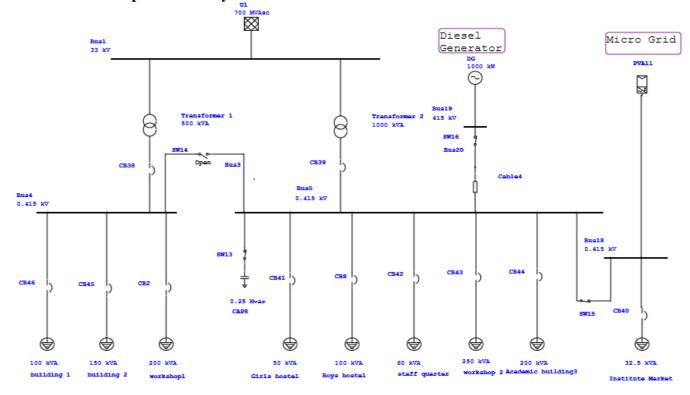
Fig. 1 Single line diagram
