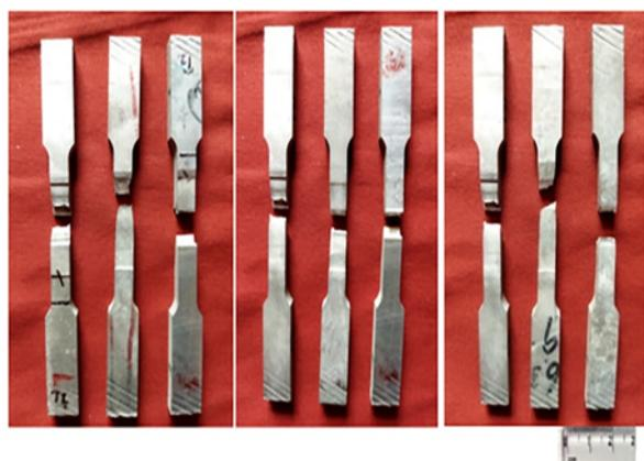
**FIGURE 2.** Tensile Failure AA6082/AA5083 Samples
