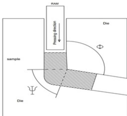
**FIGURE 1.** Four basic routes in the Equal Channel Angular Pressing process and Sample Passes through Channel.
