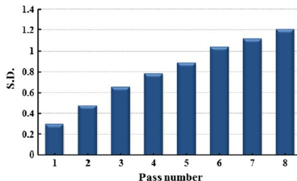
**FIGURE 3.** The average S.D. values for every pass number up to 8 passes, regardless of die channel and angles of outer corner.
