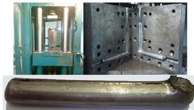
**FIGURE 2.** After one pass pressing, Equal Channel Angular Pressing die and AA5083 billet.
