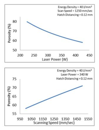
**FIGURE 3.** Effect of process parameters on porosity during SLM
