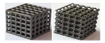
FIGURE 2. Porous Ti-6Al-4V scaffolds by SLM
