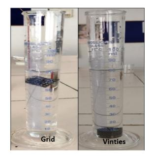
**FIGURE 4.** Porosity measurement ofscaffolds by measuring cylinder
