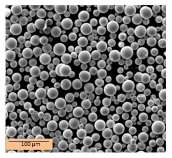
FIGURE 1. SEM morphology of Ti-6Al-4V powders
