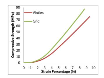
**FIGURE 6.** Compressive stress vs staincurve for the porous Ti-6Al-4V scaffolds
