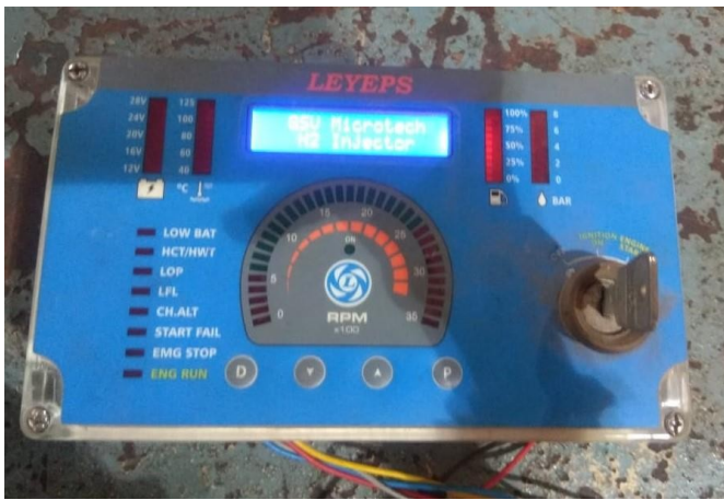
FIGURE 4. ECU to Control MEA Injection
