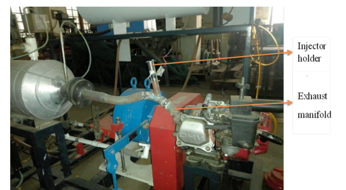
FIGURE 7. Pictorial View of Modified Exhaust
