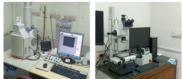
(a) Scanning Electron Microscope (b) Digital Measuring Microscope
