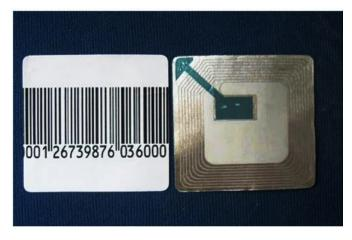
FIGURE 3. RFID Tag or Card
