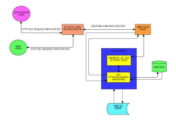
FIGURE 6. Cloud components flow diagram
