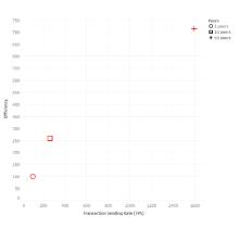
FIGURE 9. Transactions sending rate vs efficiency for different endorsement phase
