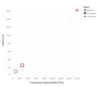
FIGURE 10. Transactions sending rate vs latency for different endorsement phase.
