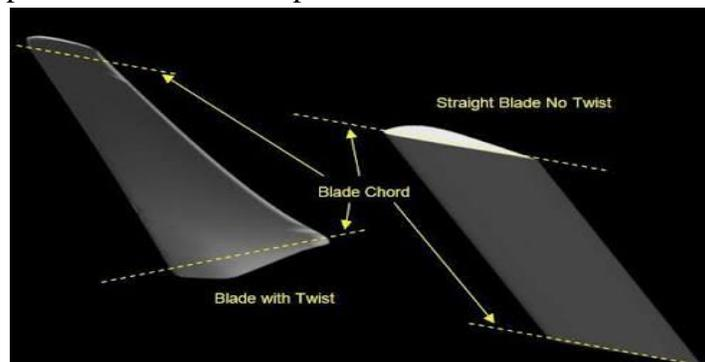
Figure.6 - twisted blade
