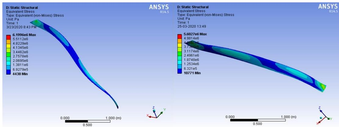
Fig.12– comparative stress analysis for aluminium and composite in case4
