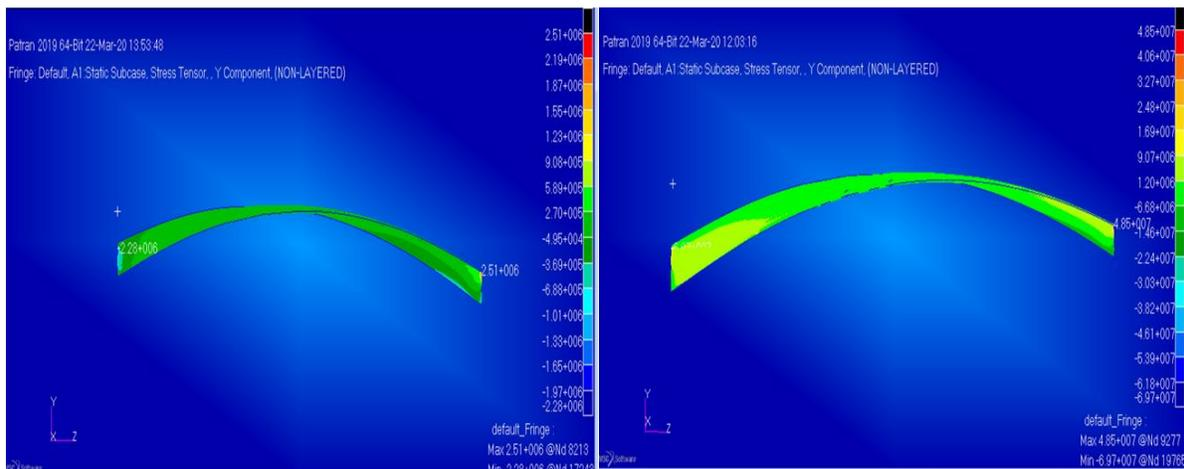
Fig.17- stress in y component for aluminium & stress in y component for composite
