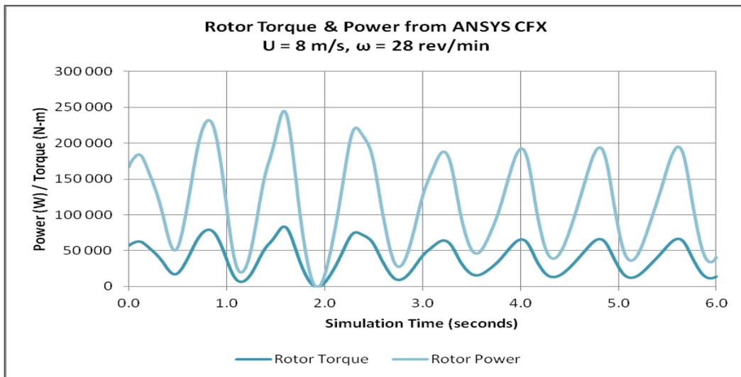
Fig.5 - Results of CFX simulation, 8 m/s wind speed
