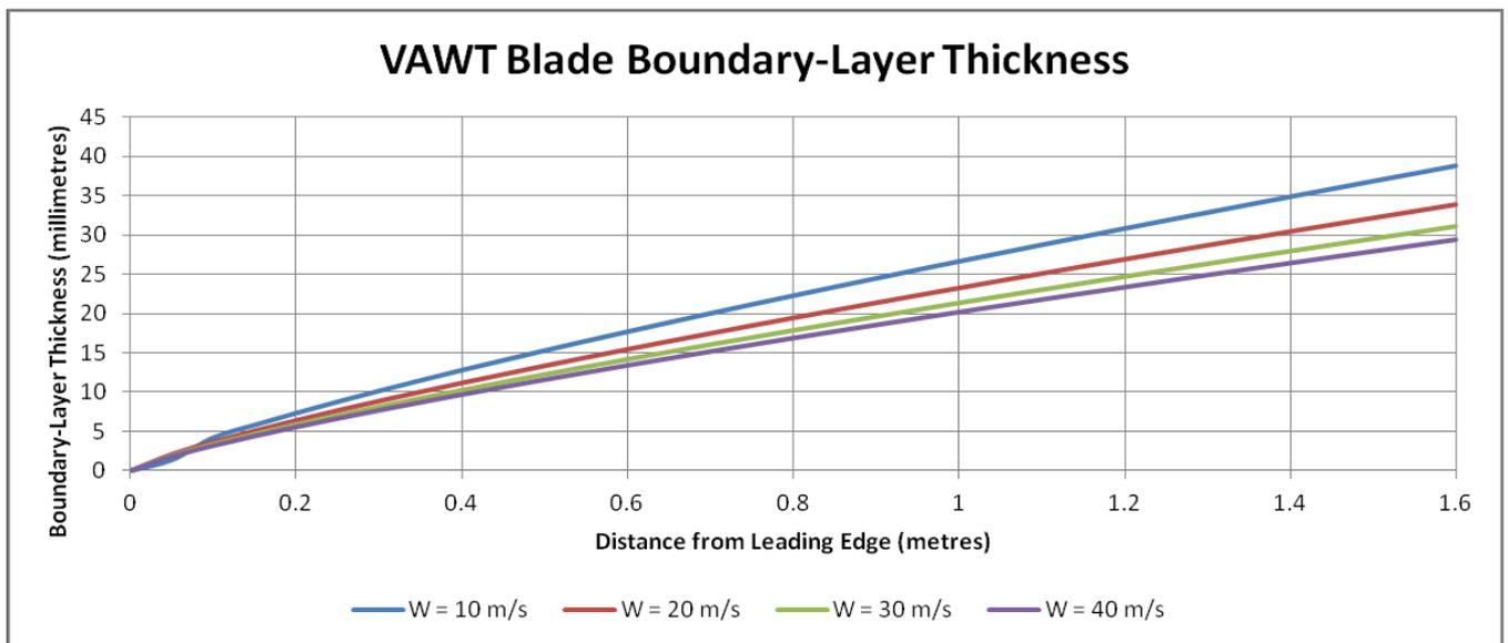
Fig.1 - Boundary-layer thickness at various stream speeds
