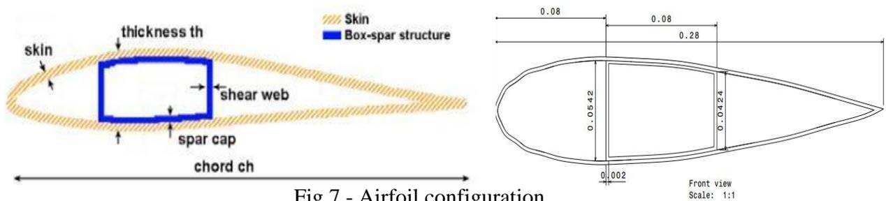
Fig.7.- Airfoil configuration
