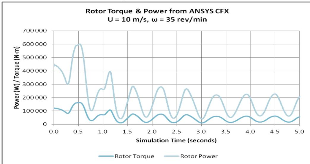
Fig.4 - Results of CFX simulation, 10 m/s wind speed
