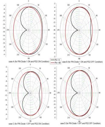
Fig.4. Radiation patterns for proposed antenna for all cases (A, B, C and D)
