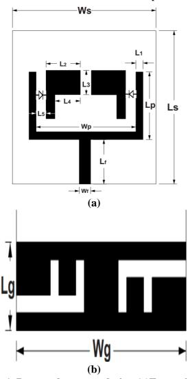
Fig.1. Proposed antenna design (a)Front view (b)Rear view
