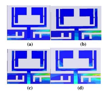
Fig.6. Surface current distribution for all the four cases were shown in (a)case A, (b)case B, (c)case C, (d)case D
