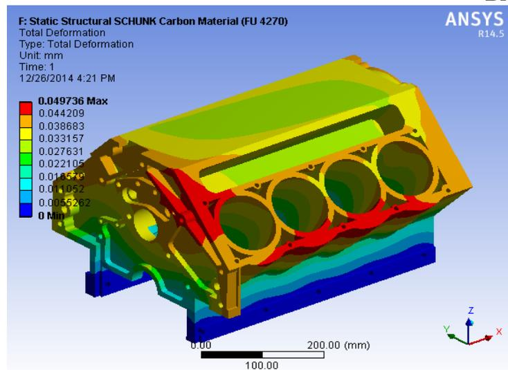
Fig.17. Total deformation for Cylinder Block for FU 4270
