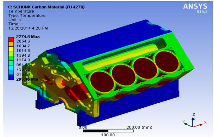
Fig.14. Maximum Temperature distribution of Cylinder Block
