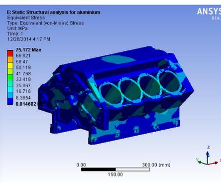
Fig.11.comparable Stress produced in cylinder Block
