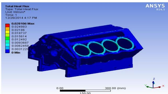
Fig.8.Steady state thermal investigation of engine Block
