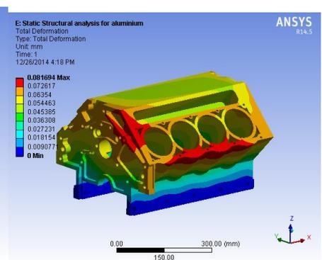
Fig.12.Total deformation produced in cylinder block
