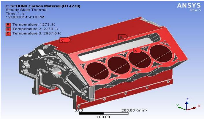
Fig.13 Temperature distribution for steady state
