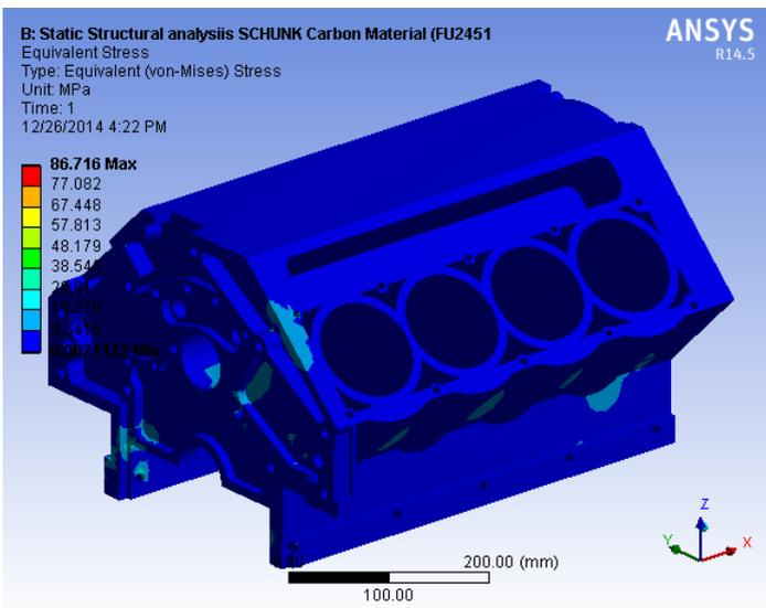
**Fig20.Equivalent Stress induced in Cylinder Block**
