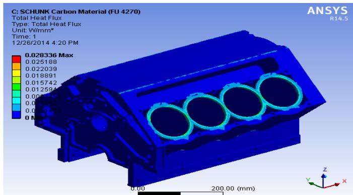
Fig.15 Heat Flux produced for FU 4270
