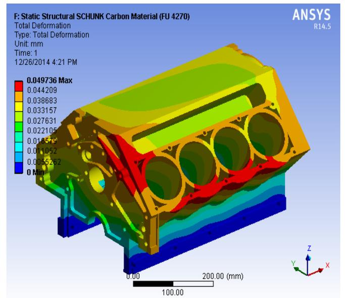
**Fig.21. Deformation induced in Cylinder Block for FU2451**
