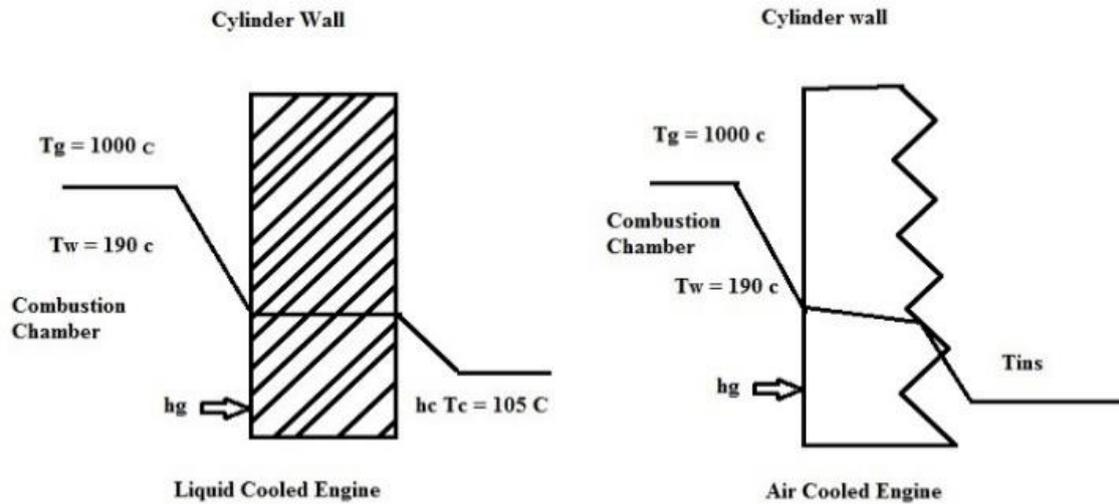
**Fig.1. Heat transfer from end to end of combustion chamber wall**
