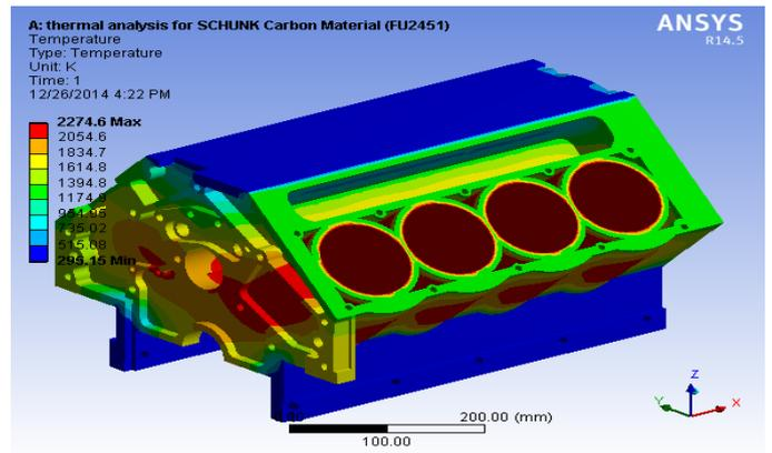
**Fig.19.Temperature circulation for Cylinder Block of FU 2451**
