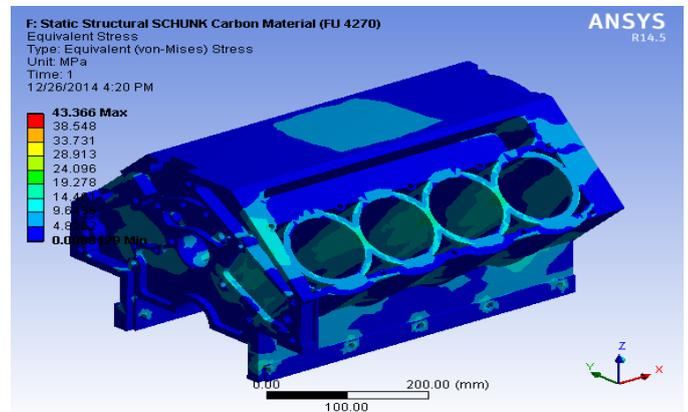
Fig.16. Equivalent stress induced in Cylinder Block
