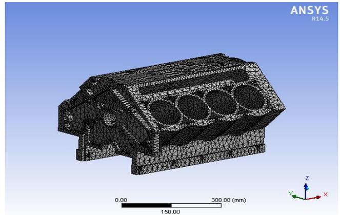
Fig.7.Discritization of the Cylinder Block
