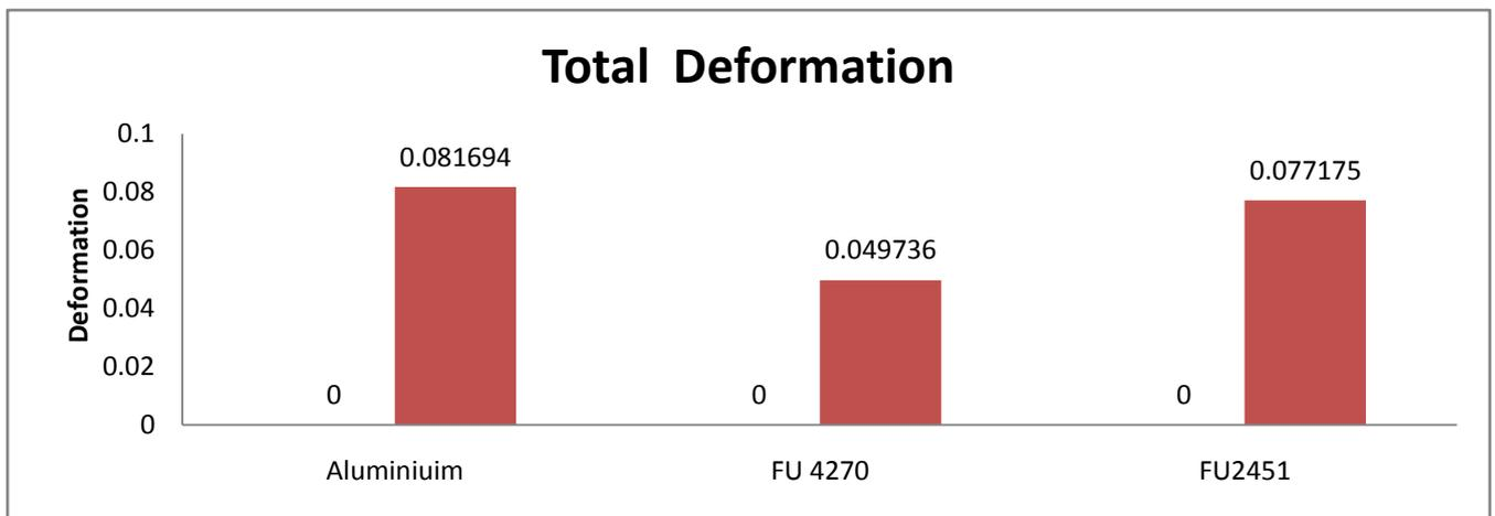
**Fig.24 Deformation comparison for Aluminium, FU 4270 and FU 2451**
