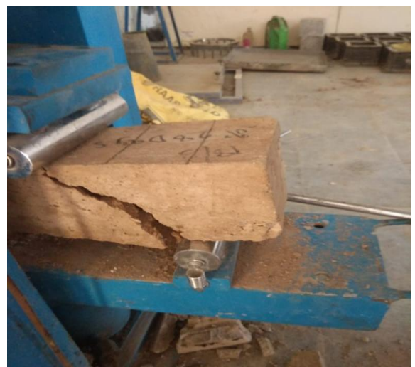
Fig.15. Tested Bamboo Reinforced sample
