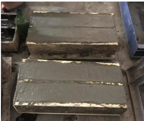
Fig.12. Casted Sample Beams
