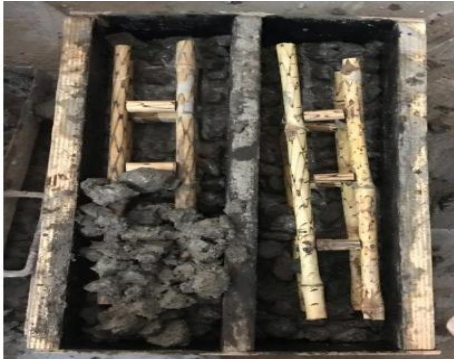
Fig.10. Sample Beam with Bamboo
