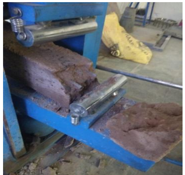
Fig.14. Tested Steel Reinforced sample
